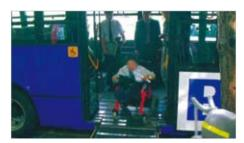
Figure 2.23 Disabled disembarking from an articulated bus in Seoul
